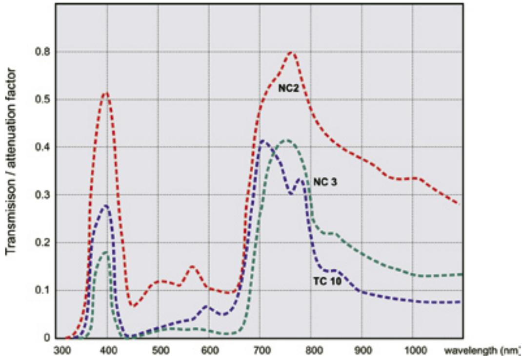
**Fig.3 - Spectral characteristics of ND filters**
